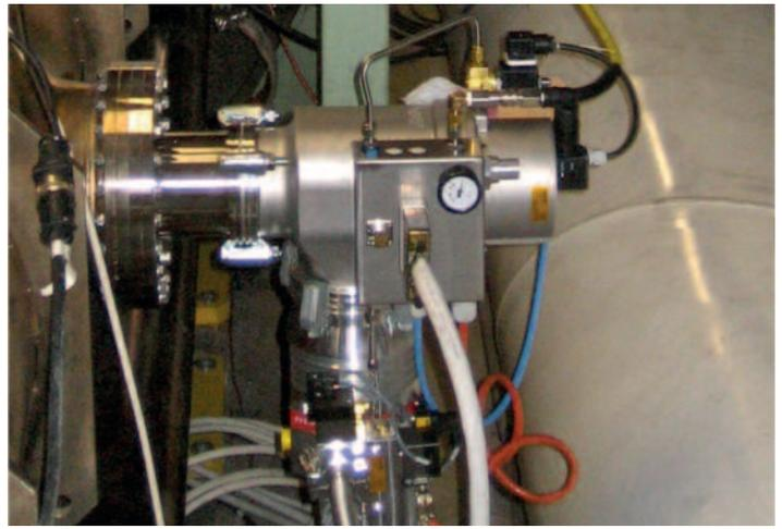
Beam vacuum generation with HiPace 300 turbopump
