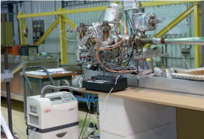
Leak testing system for LHC components with ASM Graph
