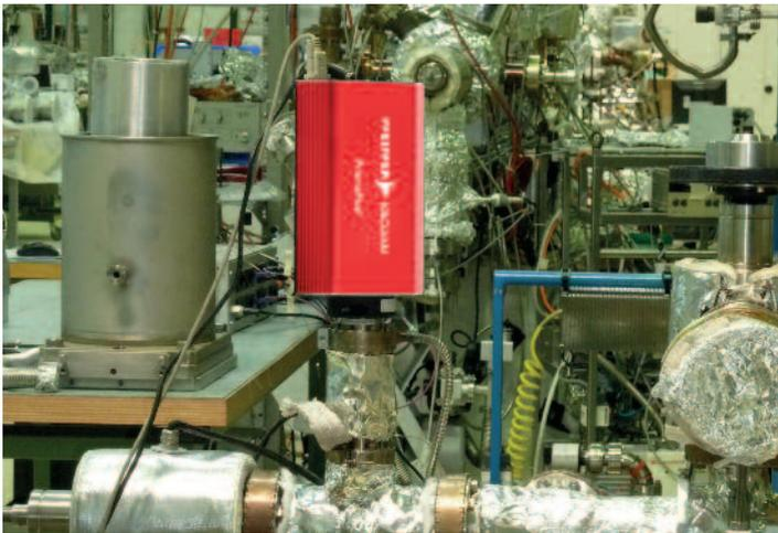
Testing system for the outgassing behavior of LHC components with PrismaPlus
