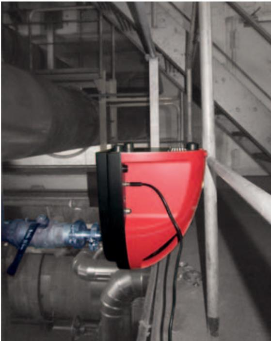
The MiniTest 300 was flanged directly to the vacuum system. Leak detection can be carried out in a radius of up to 100 m with the wireless remote control.
