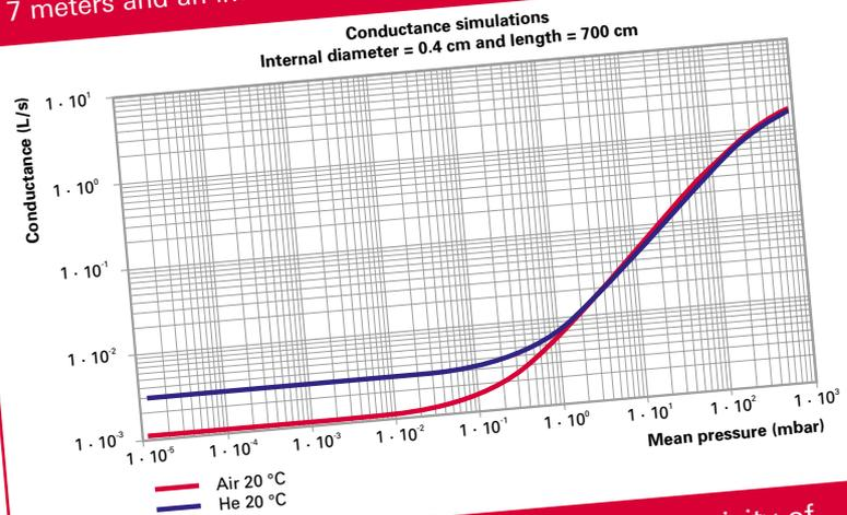
At atmospheric pressure, the pipe has a conductivity of just over one liter per second. At 0.01 mbar, the fine leak threshold of many commercial leak detectors, the same pipe has a conductivity for air of only  $10^{-3}$  l/s.
