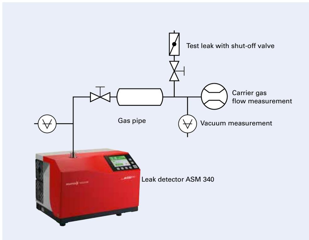
Figure 3: Helium spray test with tracer gas. An exemplary experimental setup consists of an ASM 340 leak detector with ASM View software. At both ends of each specimen, type TPR 280 Pirani tubes with a TPG 262 DualGauge measurement instrument are used as pressure gauges.
