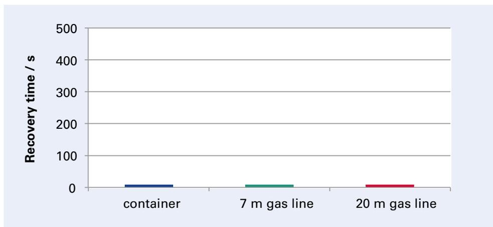
Figure 1: Recovery time without carrier gas
