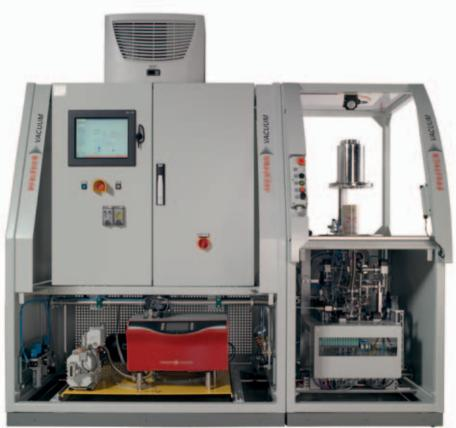
Vacuum solution for the helium leak testing of sealed cans
