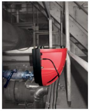
The MiniTest 300 was flanged directly to the vacuum system. Leak detection can be carried out in a radius of up to 100 m with the wireless remote control.
