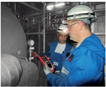
Checking the leak rate on a low-pressure pre-heater with the MiniTest 300. Measured values are indicated on the wireless remote control.
